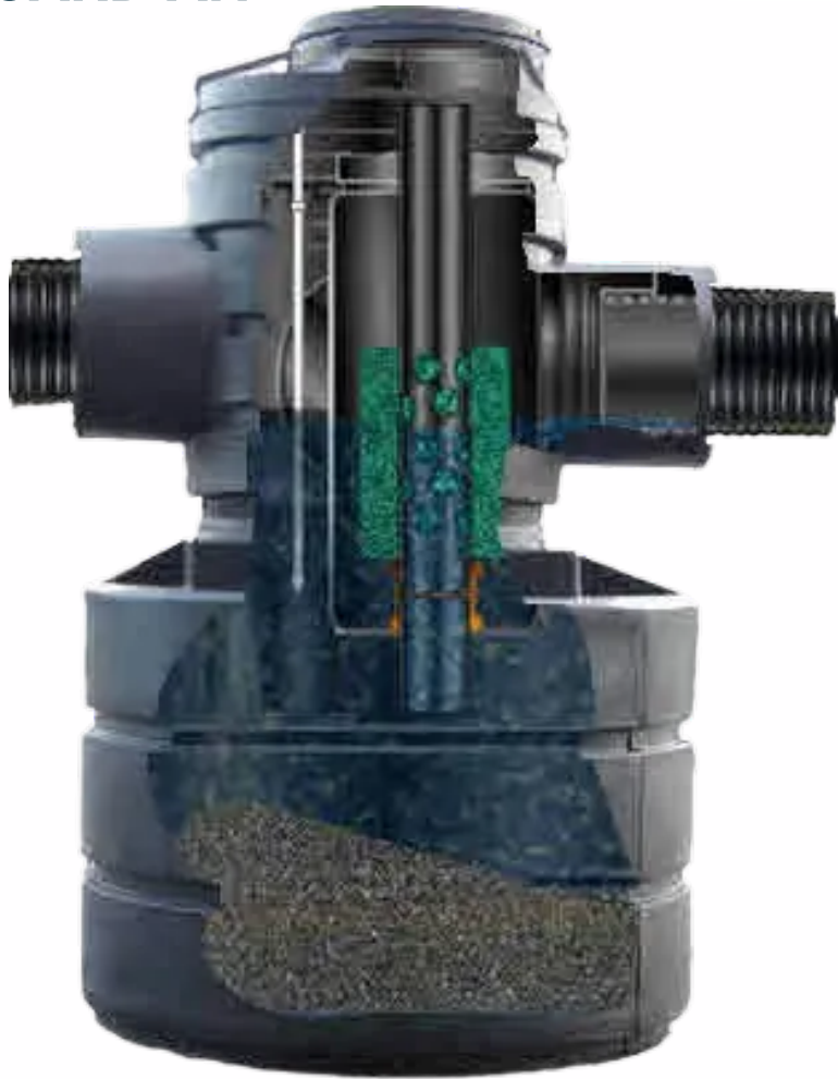
• SG 1 - Diagram showing silt retention process.
